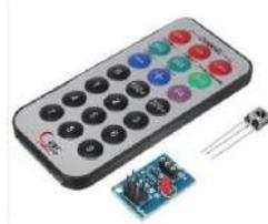
Gambar 4 Infrared Remote
