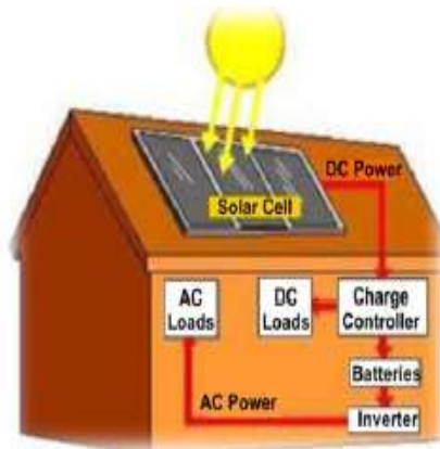
Gambar 3. KOMPONEN SOLAR HOME SYSTEM
