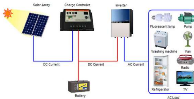
Gambar 6. RANGKAIAN LISTRIK TENAGA SUYA
