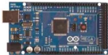
**Gambar 3.**Arduino Mega 2560
