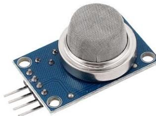
Gambar 3. Modul Sensor MQ-2 [12]
